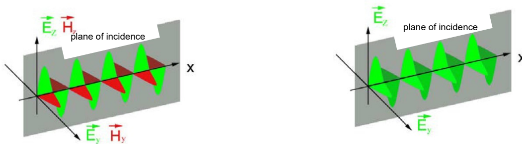
FIGURE 7: An electromagnetic wave \vec{E} \perp \vec{D} \perp \vec{k} (left); electromagnetic waves polarized in incident plane \vec{E}_z and perpendicular to the incident plane \vec{E}_y (right).
